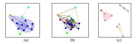
**Fig. 2.** The screenshots of the Behaviour Analytics Moodle Plug-in: (a) generating the students' behaviour graph; (b) finding the centroids of the students' behaviour graphs; and (c) clustering students in group according to the centroids of students' behaviour graphs.
